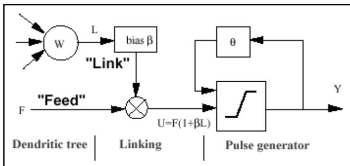
Fig. 2. The structural model of the pulse-coupled neuron
